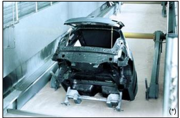
dipping of a body-in-white into an E-coating paint bath (*)
