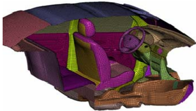
Figure 3. Section in the thermal finite-element model of the vehicle
