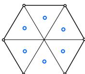
Figure 3: Gauss point distribution for Hexahedral Element.
